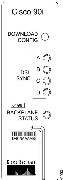
The Cisco 90i is a single-width D4 channel unit that is compatible with existing D4 channel banks, using standard common equipment. It supports four ISDN Digital Subscriber Lines (IDSLs) running user data at either 56, 64, 128, or 144 kbps. Each of the four subscriber interfaces supports standard twisted-pair 2B1Q loops of up to 18 kilofeet.
